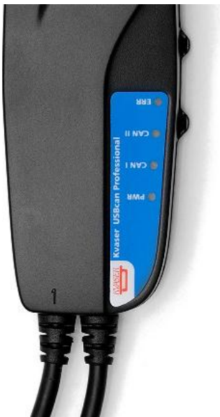
Figure 3: The CAN channels on Kvaser USBcan Professional.
