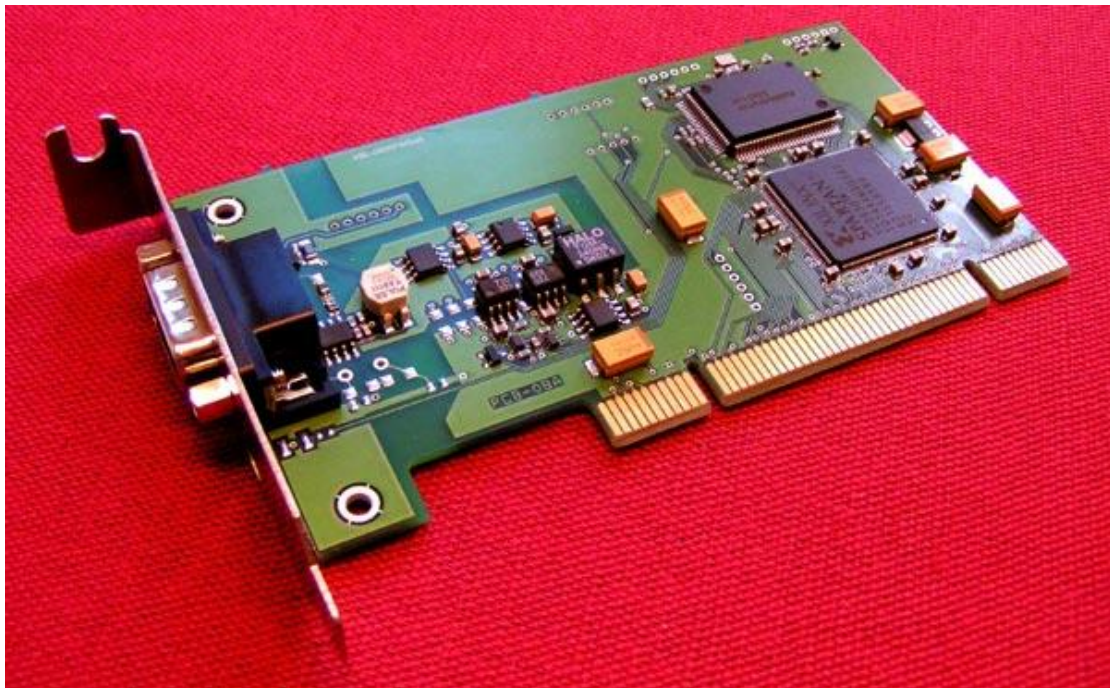
Figure 2. Kvaser PCICanx II HS with the low profile bracket mounted
