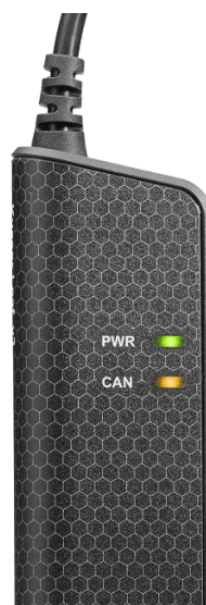
Figure 4: LEDs on the Kvaser Leaf v3 J1939-13 Type II.
