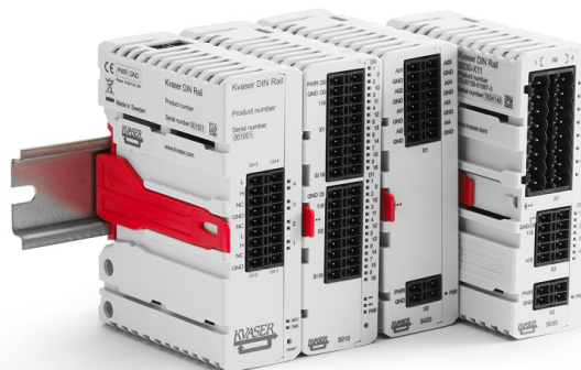
Figure 5: Mounting add-on modules to the DIN Rail.
