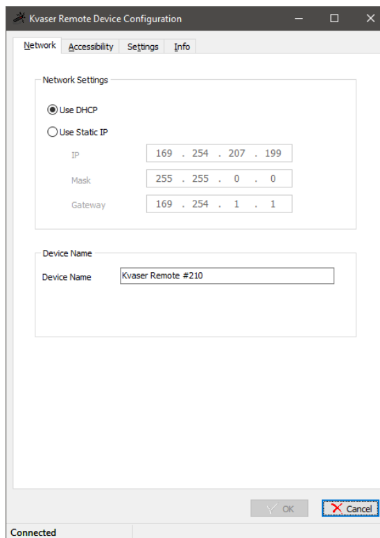
Figure 21: Kvaser Remote Device Configuration network settings
