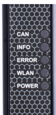
Figure 3: LEDs on the Kvaser BlackBird v2
