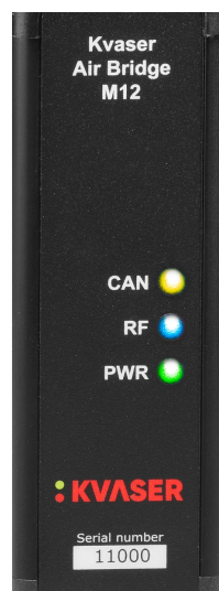
Figure 3: LEDs on the Kvaser Air Bridge M12.
