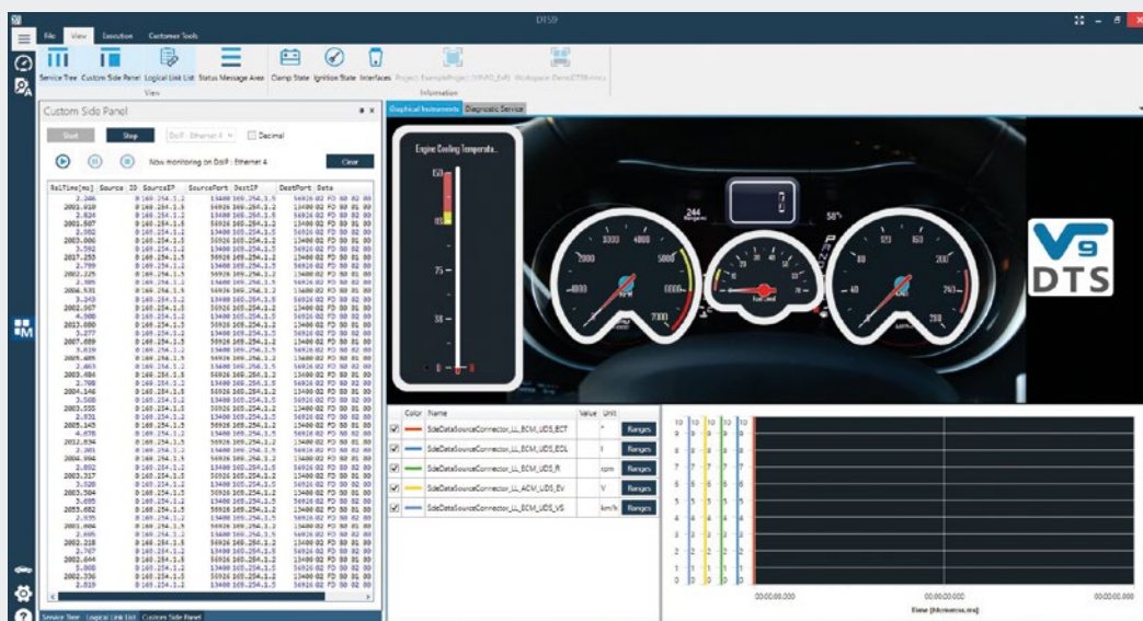
▲ Fig.: Softing DTS.monaco (Generation 9) – New Platform, Graphical Instruments and DoIP Monitor
