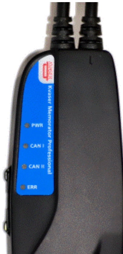
Figure 5: LEDs on the Kvaser Memorator Professional
